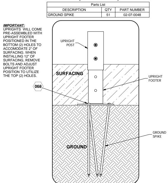
**IMPORTANT:** Never install play equipment over hard, unresilient surfaces such as asphalt, concrete, or compacted earth. It is the owner's responsibility to ensure the "minimum area required" contains an appropriate amount of resilient material to cushion accidental falls.
