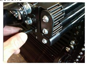
Step #1 Remove 9/16" bolt from bottom of partition
