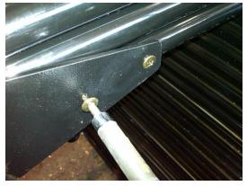
Step #4 Insert two Phillips head screws into side of caster base, and tighten with screwdriver.
