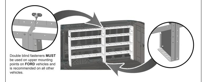
**STEP 10.** Assemble a lock washer and a flat washer to each 1/4-20 x 1-1/4" mounting bolt, and loosely attach the shelf unit to the blind fasteners in the van wall through the mounting angles. Once all brackets and mounting bolts are in place, re-check for alignement and tighten all bolts to 24 in-lbs.
