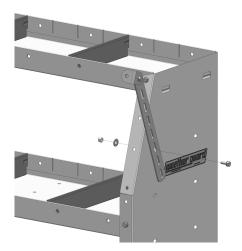
It is important to make sure that the mounting straps are attached on the end panels perpendicular to the van walls. The mounting strap needs to be bolted at two points at minimum where the strap and the end panel meets. Attach the mounting strap to end panel using a exisintng obround hole such that the strap can pivot and is long enough to reach the van wall. Use a  $1/4-20 \times 3/4$ " bolt with washer and a nylon lock nut but do not tighten at this time.
