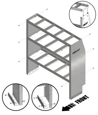
Mounting bracket should overlap and support end panel. It can be mounted on either side.
