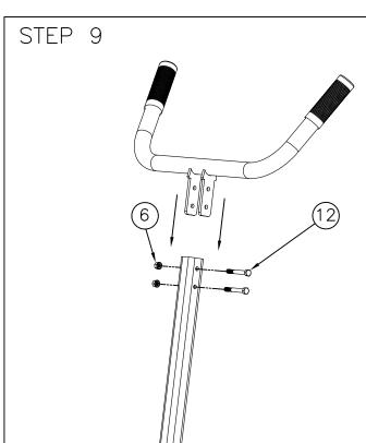
Slide handle onto post and fasten with two locknuts(6) and two bolts(12).
