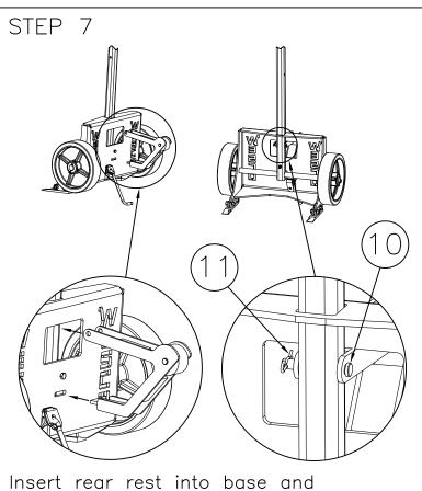
secure with clevis pin(10) and
